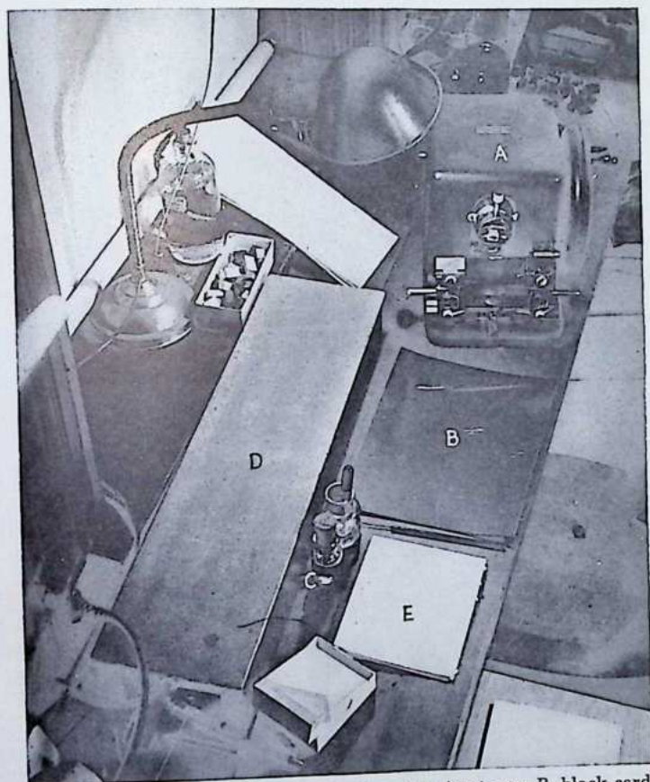
FIG. 7.—Arrangement of table for microtoming: A, microtome; B, black cardboard on which to place ribbons; C, bottles with adhesive and flooding solution; D, warming plate; E, absorbent paper towel folded over, for draining excess flooding solution. Box of slides is at one end of the warming plate. Lamp should be so placed that the light is directed in front of the microtome knife.
